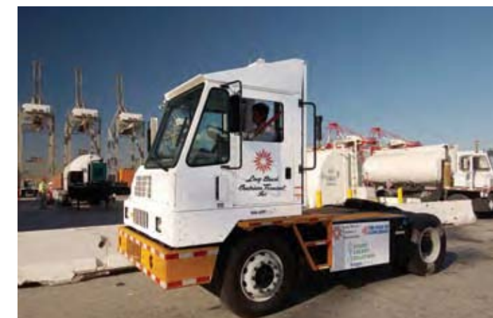
Alternative technologies, such as this LNG-powered yard hostler, are a key part of the Port's Green Port strategy.
