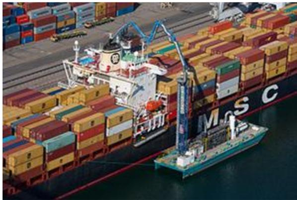
Container and cruise ships must significantly reduce at-berth emissions to meet state regulations, but the existing “shore power” option requires retrofits to each vessel. According to ACTI, the AMECS barge system can meet the state standards by removing 90 to 99 percent of harmful emissions of nitrogen oxide, sulfur dioxide and particulate matter without requiring vessel retrofits.
